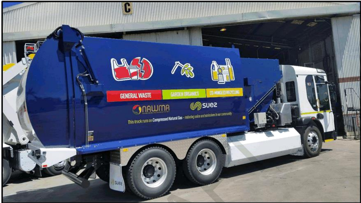
Image: Suez Truck using High Density Compressed Natural Gas as a Fuel Source
