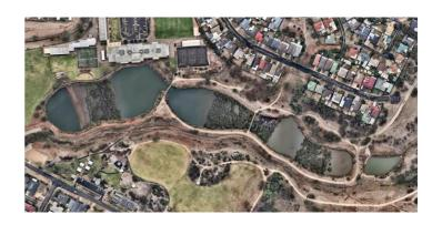
Constructed wetlands, such as Andrews Farm, are used to clean stormwater to ensure it can be recycled or discharged to the environment safely. It uses a natural process to filter and clean the stormwater and this occurs through using a number of physical, biological and chemical techniques.
