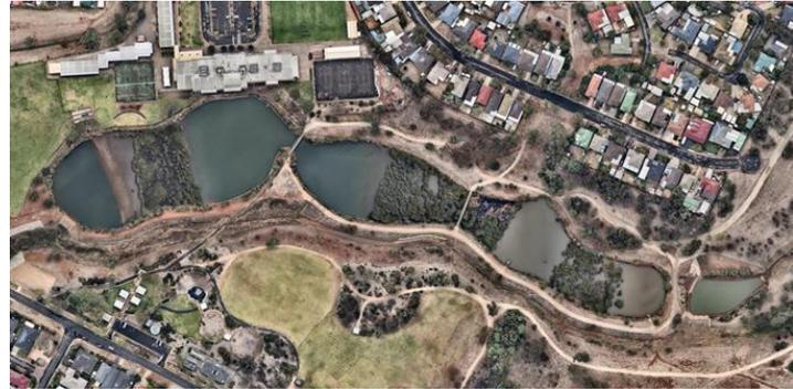
Constructed wetlands, such as Andrews Farm, are used to clean stormwater to ensure it can be recycled or discharged to the environment safely. It uses a natural process to filter and clean the stormwater and this occurs through using a number of physical, biological and chemical techniques.
