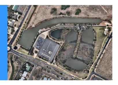
Constructed wetlands, such as Stebonheath Curtis, are used to clean stormwater to ensure it can be recycled or discharged to the environment safely. It uses a natural process to filter and clean the stormwater and this occurs through using a number of physical, biological and chemical techniques.
